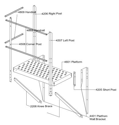
On standard 32" and 44" bin sheets the platform Wall Brackets will attach 4 bolts (37 ½") apart. Attach Wall Brackets to bin. In the lowest hole of the Wall Bracket attach Knee Braces.
